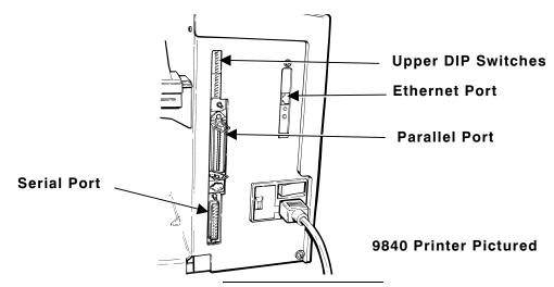
Do not plug any cables into the parallel port when using the Ethernet port.
